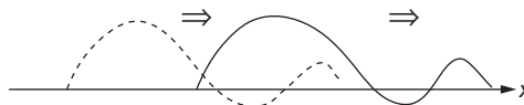
FIGURE 9.4 Traveling wave f(x - ct) . Dashed line is profile at t = 0 ; full line is profile at a time t > 0 .
